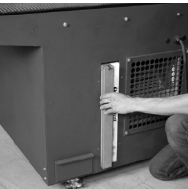
7. Replace Metal Mesh Prefilterer (if applicable).
