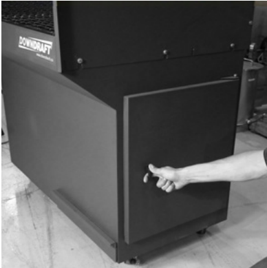
4. Inspect cabinet interior for debris.
