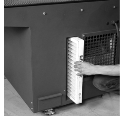
6. Ensure airflow indicator points in correct direction.
